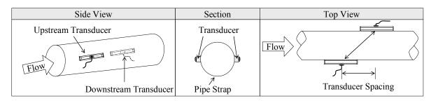
The Z method is able to measure on pipe diameters ranging from 25mm to 1200mm (1"~48") approximately.
